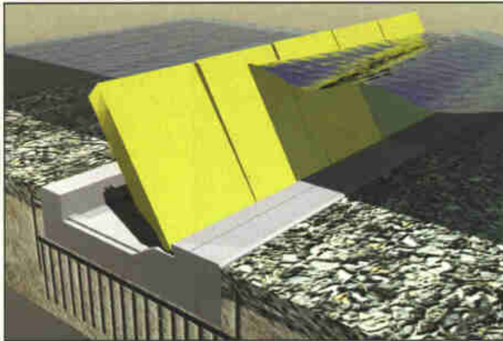
THE GATES fill with water under normal tidal conditions and rest on the inlet canal bed. When tides reach 100 cm, the gates will be filled with compressed air and rise to isolate the lagoon from the sea.
